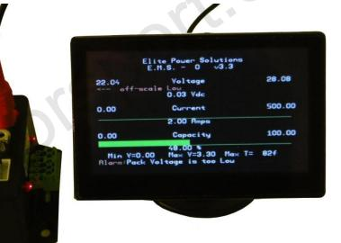
Connect the video output to a screen. The above will be displayed. "E.M.S. -0" will be displayed. This is the number of sense boards the CPU has detected.
